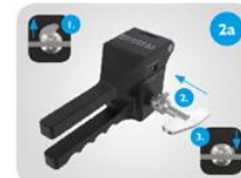
Attach turning lever to the shaft of the blade cylinder 1. Open the locking mechanism. 2. Slide the lever onto the shaft as far as it will go. 3. Close the locking mechanism.
